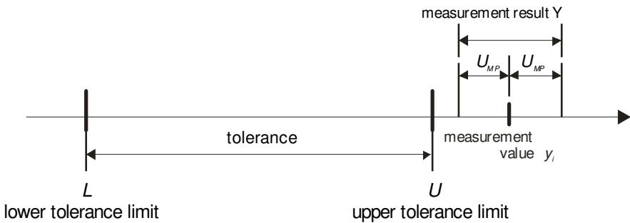
Figure 3: Proof of non-conformance with the tolerance
